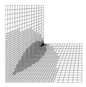
Figure 9: L-shape domain with cubic THB-splines after four adaptive refinement steps (2379 dofs)
