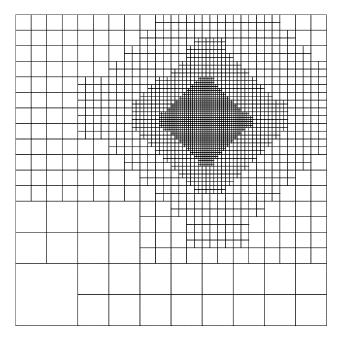
Figure 6: THB-spline supports after five steps of adaptive fitting with quadratic THB-splines (Example 1)
