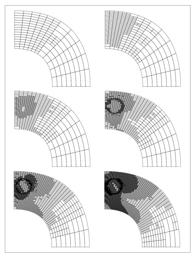
Figure 8: Meshes for different multigrid levels  $\ell = 1, \dots, 6$  in Example 2 using quadratic THB-splines.
