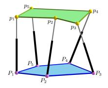
FIGURE 1. Sketch of an n-pod for n = 5, a pentapod.
